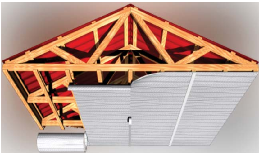
Reflective insulation can either be draped over purlins or attached to the inside.
